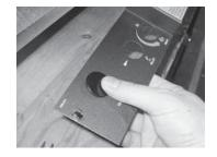
**22)** Attach the DC sparker generator connector to the valve with a screw.
